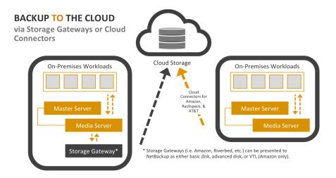
Since the cloud is a great low-cost, low-maintenance storage option, it's an attractive way to reduce IT storage costs. In this scenario, your on-premises data center runs normal backup operations and backup data is moved to the cloud via cloud connectors or a storage gateway. Data can be recovered through NetBackup's self-service portal.
