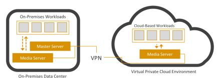
In this true hybrid scenario, you have a mix of on-premises and cloud-based workloads. The backup infrastructure and cloud-based workloads are hosted in a virtual private cloud environment using a service such as Amazon EC2 or Microsoft Azure. In this case, you'll have full visibility and control of your cloud-based workloads through your on-premises data center including quick data recovery through a self-service portal.
